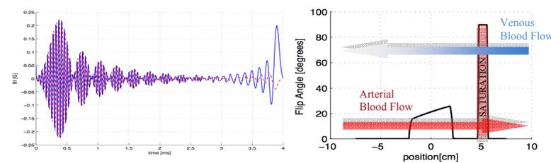
**Figure 1:** Designed RF pulse waveform (imaginary in red, real in blue) after inverse SLR transform and B<sub>1</sub> scaling for a duration of 4ms, time-bandwidth-product of 68 and the corresponding simulated pulse profile (right).
