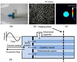
Fig. 1(a) Lateral view of the phantom, (b) microscopic image of imaging plane, (c) acquired ADC image in a state of rest, and (d) phantom for simulating that the water fluctuation was affected by biomechanical factors.
