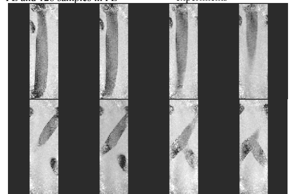
Fig. 6. Resulting sagittal ADC maps showing the fiber tracks. Slice thickness = 2.8 mm, FOV in PE was reduced to 4 cm and TE to 88 ms. Resolution matrix = 32×128 (PE×FE). Total number of bands excited = 20. Aliasing from imperfect suppression of signal outside the bands is very weak.
