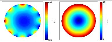
Figure 1: Center slice B<sub>1</sub><sup>+</sup>(left) and |E| (right) fields; averaged over all three simulations. Each single field pattern closely agrees with the shown average.
