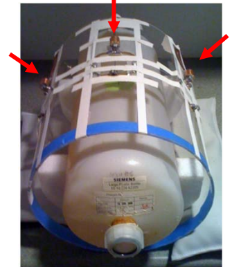
Figure 1. The cylindrical agar gel phantom having conductivity of 0.77 S/m and permittivity of 58. The three transmit/receive coils were located under the phantom (see red arrows).
