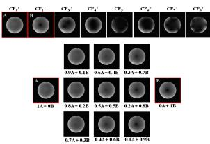
**Fig 2**: GRE sugar/water phantom. **Top row**: images generated by  $CP_1^+$  mode and clockwise higher CP modes. **Remaining rows**: to estimate the optimal image combination, selected combinations of weighted  $CP_1^+$  mode (A) and  $CP_2^+$  mode (B) were generated.
