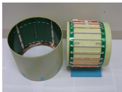
**Fig. 1.** Inductive birdcage and its shield.
