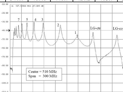
**Fig. 2.** Modes of the 24-mesh resonator.
