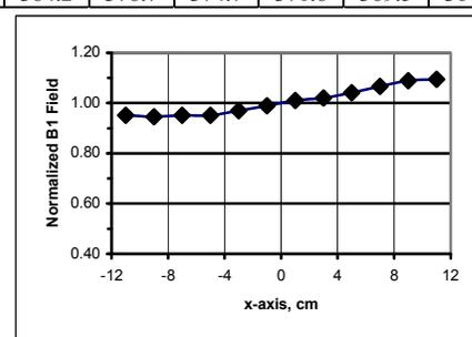
**Fig. 3.** B1 plot of the linear y-polarization.
