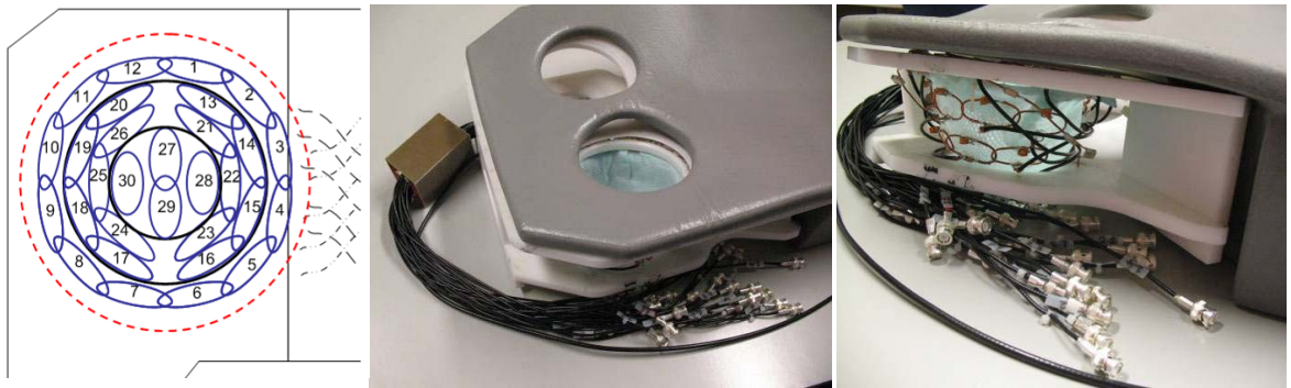
Figure 1: Schematic and photograph of the 30 channel receiver coil combined with a local transmit coil and integrated in a commercially available mechanical breast coil setup (Machnet BV, Maarn, the Netherlands). The receiver coil elements have an elliptical size of 5 by 2 cm and are decoupled using preamplifier decoupling. The entire setup is interfaced to a 7T whole body MR system (Philips, Cleveland)
