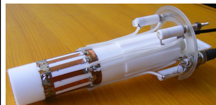
Figure 1: Mouse transceiver coil used in [6], simulated as arrangement A. Coil is a copper foil birdcage mounted on a Teflon tube, with tuning components and solder attached.
