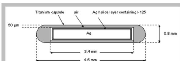
Fig. 1. Schematic representation of a brachytherapy seed, depicting the silver (Ag) core surrounded by the titanium capsule and ends.
