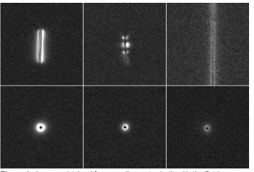
**Figure 1**: Images obtained from a saline water bath with the flat loop (left), opposed solenoid (middle) and dipole antenna (right) designs. Coil sensitivity is demonstrated along the probe (upper) and perpendicular to the probe (lower). Window and leveling are preserved between all scans.
