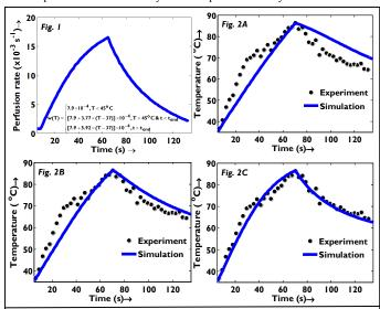
Fig. 1: Perfusion rate vs time. T is temperature, t is time and t<sub>end</sub> is the time when sonication was stopped. Fig 2: Temperature evolution at cell center were plotted using model 1 of constant thermal conductivity and perfusion rate (Fig. 2A), model 2 of temperature dependent thermal conductivity and constant perfusion rate (Fig. 2B) and model 3 of constant thermal conductivity and temperature dependent perfusion rate (Fig. 2C) and corresponding HIFU experimental data.
