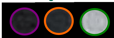
Figure 1: T1-weighted MR image of Gd-SWCNTs prepared in 4% gelatin (green), Magnevist (orange) and only 4% gelatin (purple). MR signal is enhanced by the addition of 0.2mM [\text{Gd}^{3+}] of Gd-SWCNTs as compared to Maanevist.
