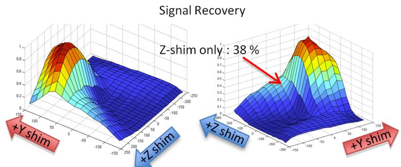
Figure 4. Signal recovery distribution along YZ-shim plane for the same slice as Fig 3.
