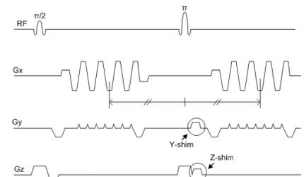
Figure 2. Pulse sequence diagram for the dual echo YZ-shim EPI sequence. The arrows denote the Y-shim and Z-shim gradients to compensate for susceptibility-related field inhomogeneity before an asymmetric spin-echo.
