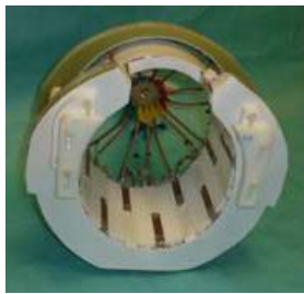
Fig. 1: Shows the 2x8 element z-encoding transceiver coil. The opening on top allows for task presentation within a head gradient coil.
