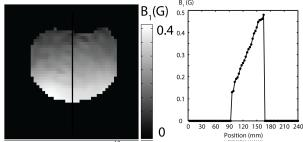
**Fig. 3.**  $B_1$  map acquired on a HP  $[1-^{13}C]$  pyruvate phantom. The surface coil is at the bottom of the image; a cross-section through the  $B_1$  map is shown. The transmit  $B_1$  falls off with increasing distance from the coil.
