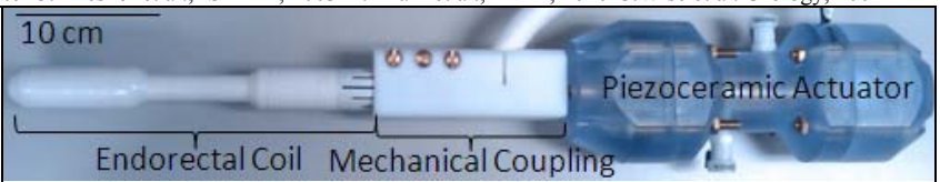
Figure 2: Picture of piezoceramic actuator mechanically coupled to the endorectal coil.
