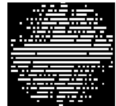
Fig. 1. CS-SENSE sampling pattern. Points in white are the sampled PE steps.
