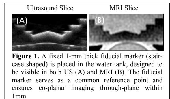
**Figure 1.** A fixed 1-mm thick fiducial marker (staircase shaped) is placed in the water tank, designed to be visible in both US (A) and MRI (B). The fiducial marker serves as a common reference point and ensures co-planar imaging through-plane within 1mm.
