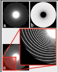
Figure 1: Example trajectory (a) and trajectory complement (b). The complement is density corrected by considering sampled points on the trajectory as well as points that will be synthesized during iterative parallel reconstruction, which lie off of the trajectory (c).
