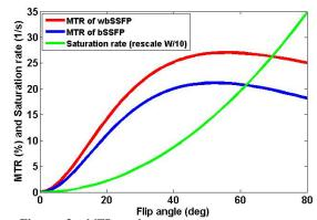
**Figure 2**: MTR and mean saturation rate as a function of flip angle, for wbSSFP and bSSFP.
