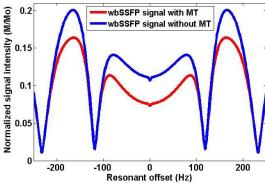
**Figure 1**: Simulated white-matter wbSSFP signal as a function of resonant offset with and without consideration for MT effects.
