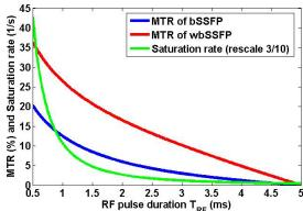
**Figure 3**: MTR and mean saturation rate as a function of RF pulse duration with fixed (TR+TRs- $2T_{RF}$ ) for wbSSFP and fixed (TR- $T_{RF}$ ) for bSSFP.
