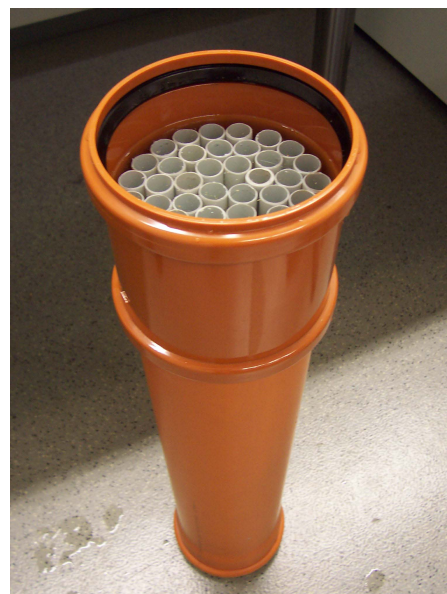
FIG 1: Structure phantom consisting of 43 tubes of 13mm in diameter.
