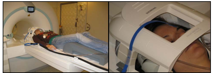
Fig. 1: Setup of the tracking system and fixation of the tape on the headcoil and on the volunteer's head.
