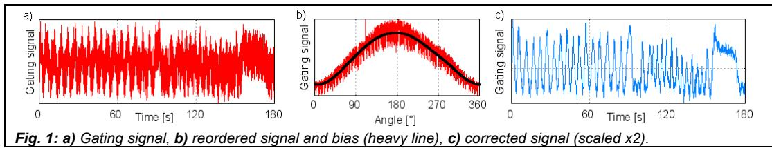
Fig. 1: a) Gating signal, b) reordered signal and bias (heavy line), c) corrected signal (scaled x2).
