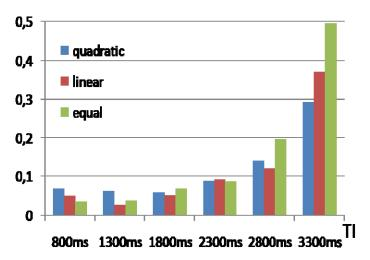
Figure 2: relative noise of the different imaging modes over TI
