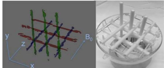
**Results Fig 2** shows the  $b_0$  images of the phantom rotated in the x-z plane, with the angle of the z-phantom wrt the scanner's z-axis. The phantom was rotated in a similar fashion in the other two planes.
