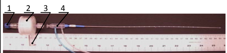
Figure 2. Laser ablation MRE driver setup. 1: connect to laser source; 2: acoustic piston driver; 3: connect to acoustic source; 4: laser applicator
