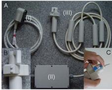
Figure 2: A: Complete needle guide with standard coil plug (I), connectable into the MR front-end, interface box (II), hand piece (III) and cabling.
