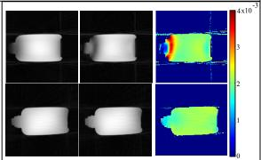
Figure.2 In the phantom experiment with the 3D radial FSE-based sequence, two scans were performed without (first row) and with (second row) the SPLICE technique. The first and the second columns are the diffusion images acquired with b=14s/(mm²) and b=351s/(mm²), respectively. The third column shows the ADC maps. The color scale on right is in units of mm²/s
