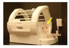
Figure 1. <sup>31</sup>P Birdcage Coil with <sup>1</sup>H Loop Coil indicated by arrow.
