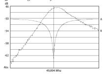
Fig. 3. Decoupling measurements: Reflection curve from the <sup>31</sup>P channel (A) and transmission to
