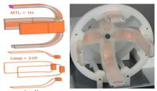
Fig. 1. <sup>1</sup>H-<sup>31</sup>P helmet coil prototype.
