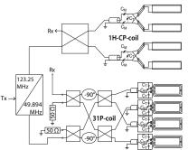
Fig. 2. Wiring scheme of the coil.
