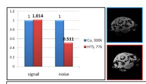
Fig. 2 Signal/noise comparison acquired by different coil settings (left). One of the images was also displayed at the right.
