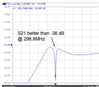
Fig. 2 Bench test result. The intrinsic decoupling phenomenon led to S21 better than -36 dB at resonance frequency.
