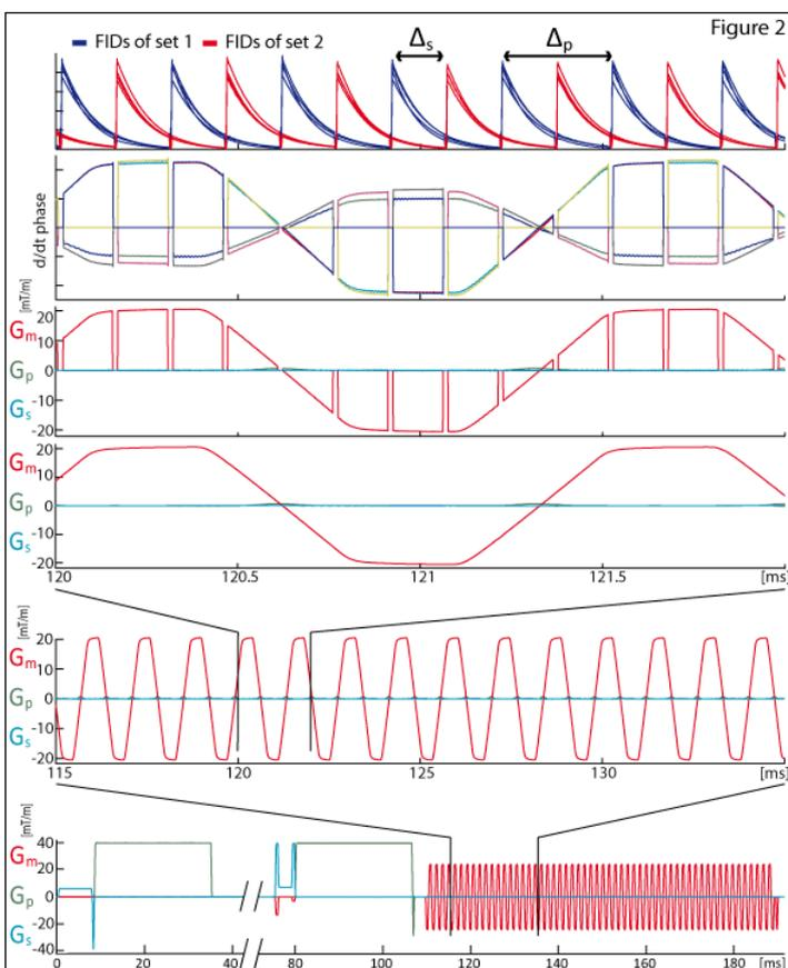
of  $1/13\mu s = 76$  kHz. The zoomed part of Fig. 2 shows some of the involved processing steps (top-down: magnitude of the FIDs, probes' field evolutions, the gradients within each time frame and the interpolated result). The measured probe SNR is in the range of 1200 at an acquisition bandwidth of 1 MHz, yielding a field resolution of 12 nT according to Ref. [1].
