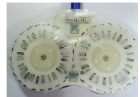
Figure 1: TMS-coil with shim. The steel for the shim was distributed as follows: Evenly along two rings around each side of the TMS-coil with a mean diameter of 70mm and a width of 10mm (each ring: 1080 mm 2 foil or 0.21 g steel), on the entrance point of the lead about 0.14 g of steel
