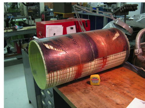
Fig 3: The innermost winding of the Z coil is shown with the thumb prints for the Y axis during mounting.
