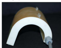
Fig. 3: Coil housing shaped for the minipig's knee
