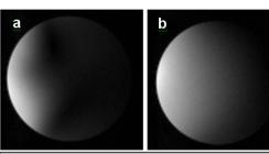
Figure 2: Gradient echo images of water phantom using linear (a) and quadrature (b) modes; TE/TR = 4/350 ms; 2 x 2 cm FOV.
