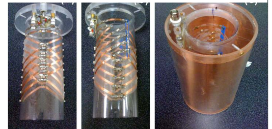
Fig. 3 Picture of ODS coil implementation. (a) View of the matching network and virtual ground points (b) Side-on view showing the orthogonal windings and (c) ODS coil inserted into the shield.
