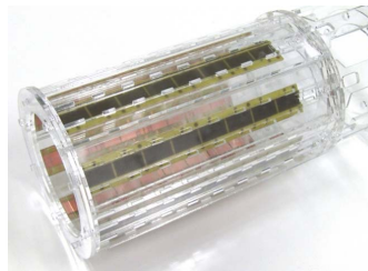
Fig. 3 Coil consisting of eight MTL elements.
