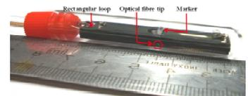
Figure 1b: MRI-Optics endoluminal probe used during our experiments.
