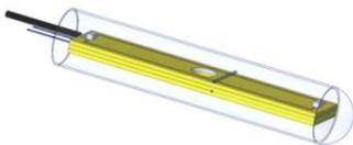
Figure 1a: Bimodal probe designed using Solidworks.
