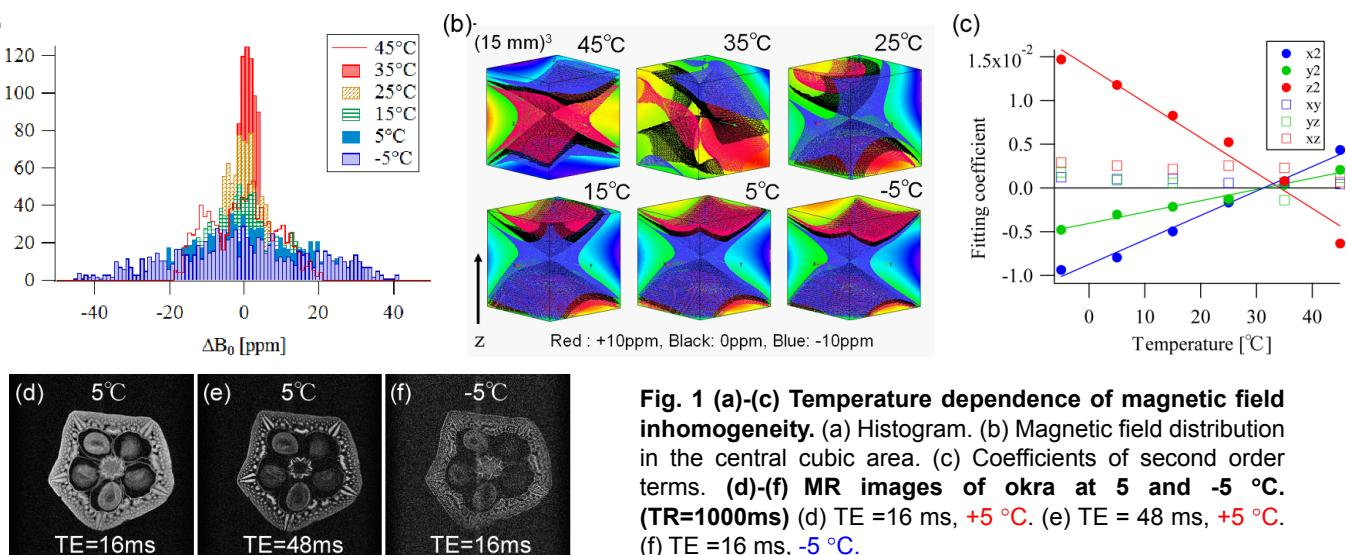
**Fig. 1 (a)-(c) Temperature dependence of magnetic field inhomogeneity.** (a) Histogram. (b) Magnetic field distribution in the central cubic area. (c) Coefficients of second order terms. **(d)-(f) MR images of okra at 5 and -5 °C.** (TR=1000ms) (d) TE = 16 ms, +5 °C. (e) TE = 48 ms, +5 °C. (f) TE = 16 ms, -5 °C.
