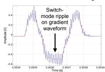
Fig 3. The switch-mode ripple
