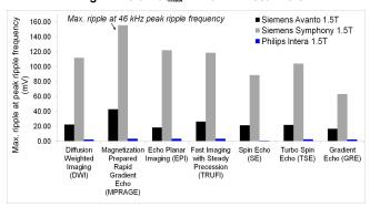
Fig 4. The maximum ripple voltage at peak ripple frequency
