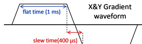
Figure 1: PNS pulse sequence
