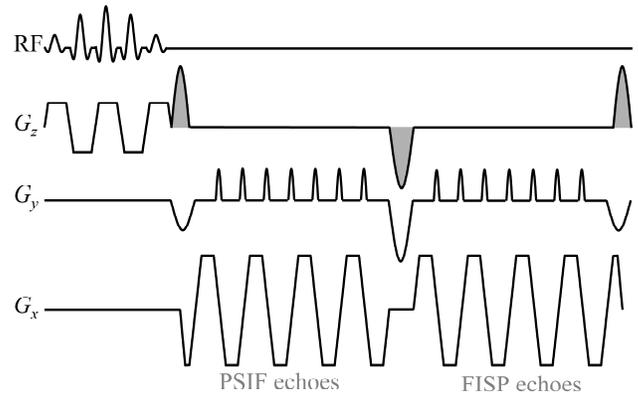
**Fig. 1:** The sequence proposed here is an interleaved-EPI sequence that samples both a FISP and a PSIF signal.
