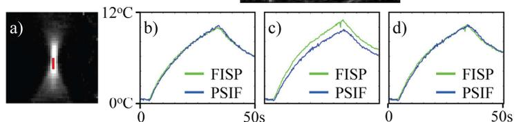
**Fig. 4:** a) Region around focus, 9x9cm. An ROI with 4 hottest voxels, shown in red, was used to generate plots. b,c) After and before high-order shimming, respectively. d) Corrected version of (c),  $\Delta TE = 1.3ms$ .
