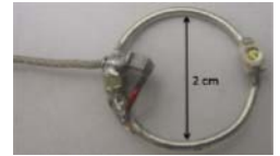
Figure 1: Local cardiac coil. It includes one tuning capacitor, one matching capacitor, and one PIN diode in series with a small hand-wound inductor for active decoupling.
