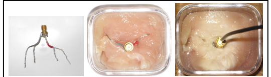
Figure 2: Ablation electrode (left) and chicken before (center) and after (right) ablation. The region around the electrode is cooked while the edges remain raw.
