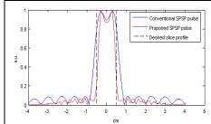
Figure1. The slice profile at 0Hz off-resonance frequency. The proposed pulse shows superior slice selectivity compared with the conventional design.
