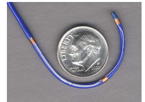
Figure 2: 5 French catheter with three integrated tracking coils.
