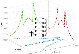
Figure 1 Coil geometry and its theoretical sensitivity profile projections along the 3 dimensions.
